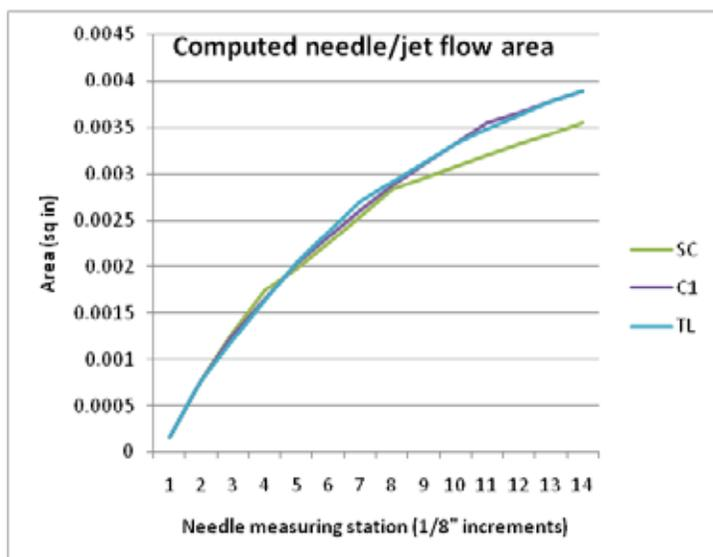
The SC needle gives the same flow area as the TL until the piston lift is about 1".
